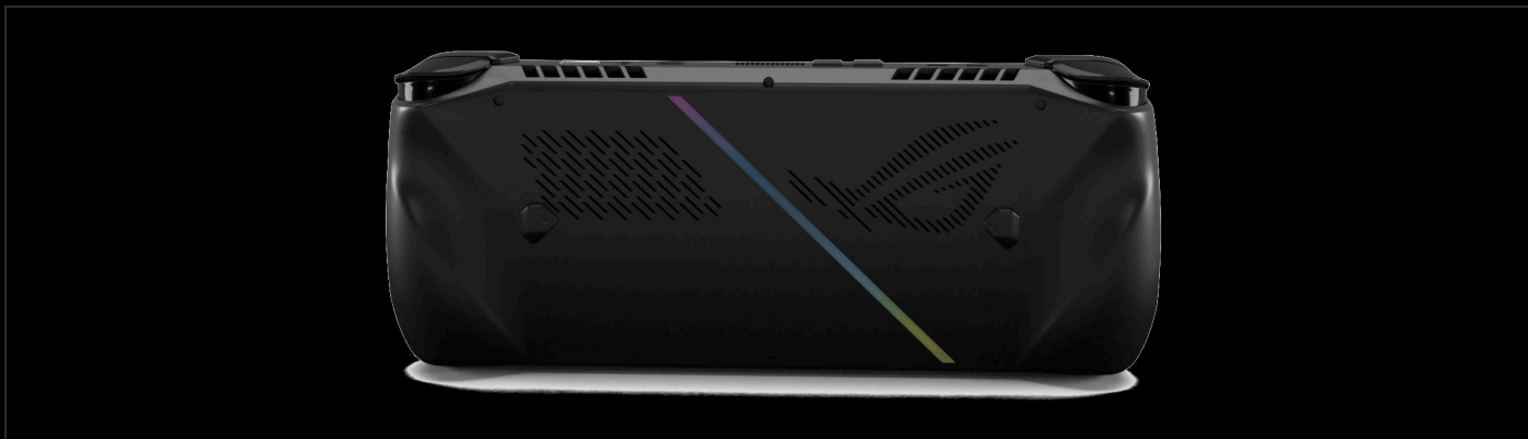
REAR CHASSIS – SIX SCREWS UNDER THE BOTTOM COVER REVEAL THE USER-SERVICEABLE SSD AND BATTERY
